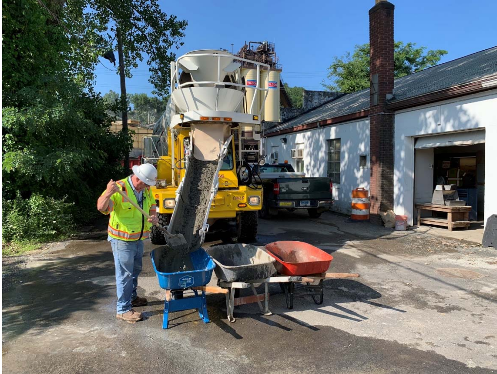
Figure 3 - Sample collection into three wheelbarrows. Each tester used independent samples.
