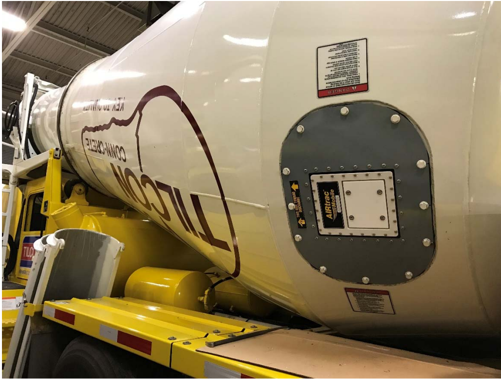
Figure 1 - SMARThatch system with integrated AIRtrac acoustic technology sensor installed on mixer drum
